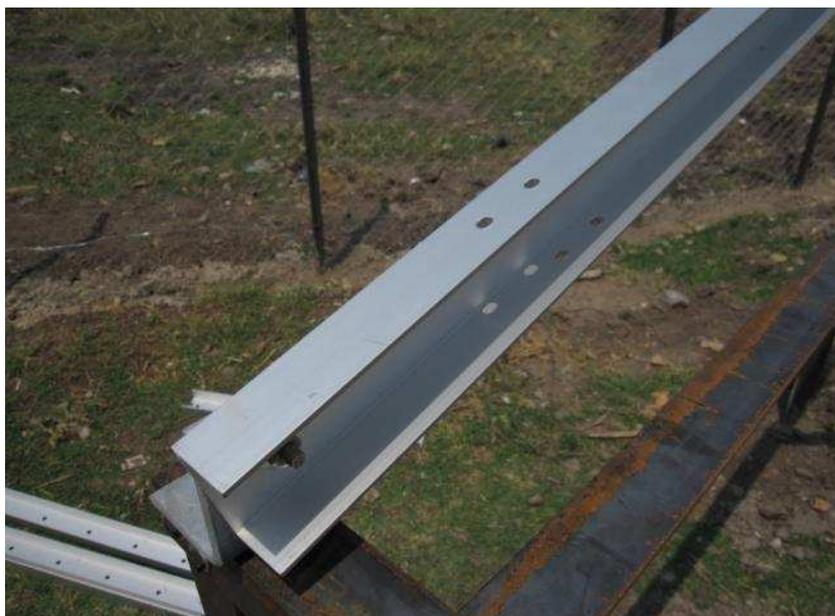
*The slightly offset holes in the support girders.*
