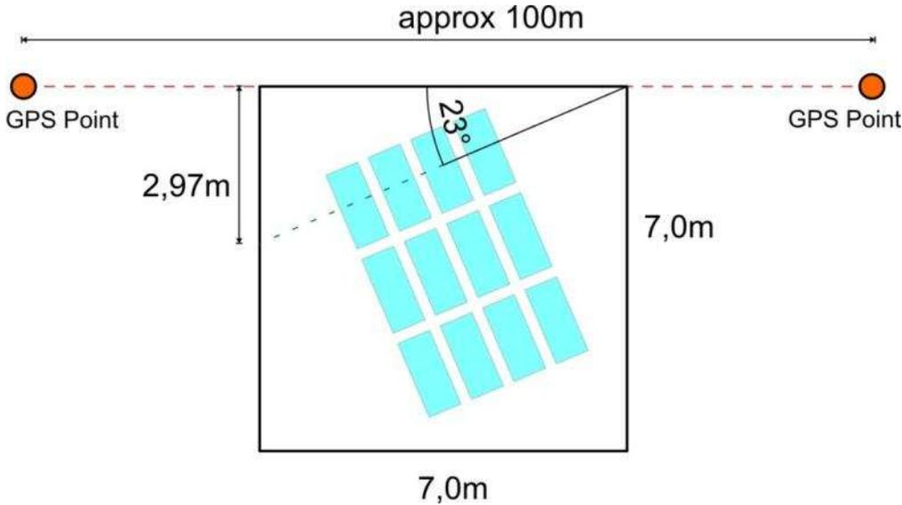
*Illustration showing how the solar panels were aligned to become properly oriented to the east.*
